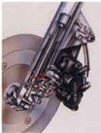
Honda's exclusive Torque Reactive Anti-dive Control (TRAC) reduces fork compression during braking.
