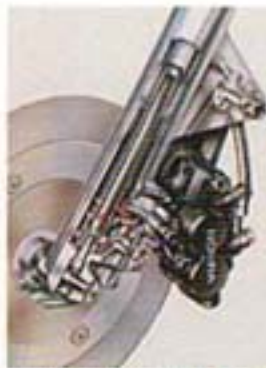
Honda's exclusive Torque Reactive Anti-dive Control (TRAC) reduces fork compression during braking.
