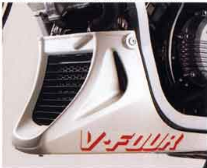
A special twin-radiator system is used to reduce frontal area and enhance mass centralization.
